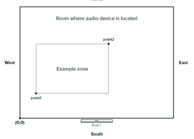
When interpreting the zone position coordinates, the origin (0,0) is the southwest corner of the room. Positive x values are in the east direction. Positive y values are in the north direction.
